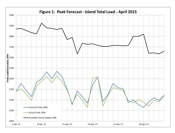
The accuracy of the forecast peaks was good for the month of April with a range of 4.5% below the actual peak to 4.0% above the actual peak. On several days the forecast peak essentially matched the actual peak; on the worst day it was 63 MW too low. On average, the forecast peak was 30 MW different than the actual peak, or 2.4%.
